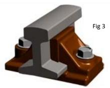
3. Place smaller section of the chair into place against the rail. Screw loosely as Fig 1 both screws will be fully tightened once the required gauge is achieved.
