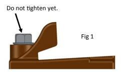
1. The chairs should be positioned on and screwed to the sleepers loosely. They will be tightened later when the gauge is set. The larger part of the chair should be on the inside edge of the rail, so that the rail cants in at 3 degrees. This is to match the coning of the wheels on the rolling stock. Enough sleepers and chairs should be assembled to take a full 4 meter length of rail at the recommended sleeper spacing of 300mm / 12" between centres.
