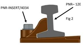
2. Install the rail to the length of sleepers and chairs that have pre assembled as Fig 1.
