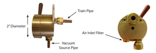
• The valve has pilot porting to aid smooth control and incorporates a sprung loaded detent to lightly locate LAP and primary positions. Full OFF and ON positions are controlled by a limit pin. The working faces of the valve are pressure pre-loaded by a disc spring, thus ensuring an airtight seal.
