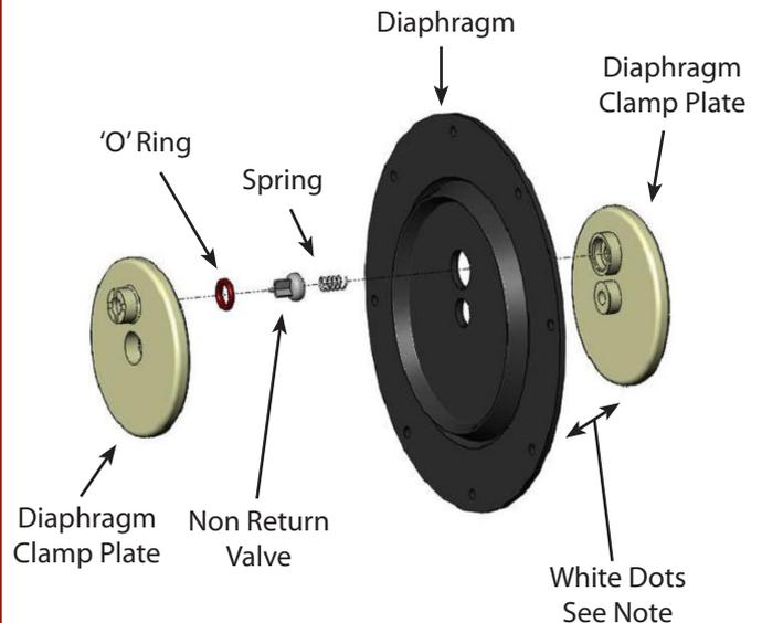
**Important Note:** Ensure that the white dots on the diaphragm and the mating clamp plate are assembled facing each other and are at this position.
