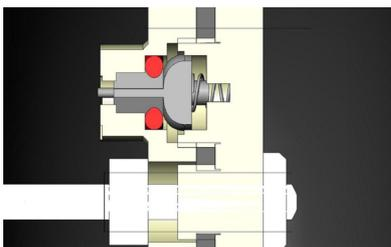
Diagram shows valve open in forward position
