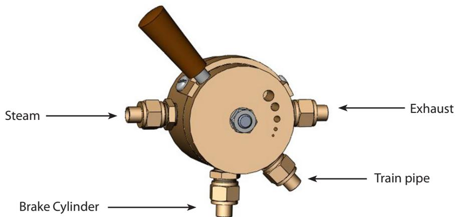
The diagram above applies to both sizes of valve and shows the functions of the ports. The smaller valves union nuts and nipples take ½" pipe and the larger valves fittings take ¾" pipe. Appropriate fittings are supplied with each valve, nipples should be silver soldered to pipes. Should the valve require maintenance contact PNP Railways.
