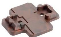
**3 Degree cant Sole Plate** - This sole plate has 3 degrees of cant to enable the rail to match the angle of the wheel coning on the wheels of locomotives and rolling stock in 7 1/4" and 10 1/4" gauge. The angle should improve running by minimizing flange contact (squealing) and hunting (side to side movement).
