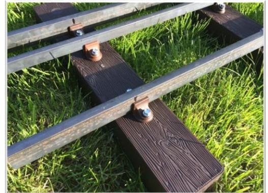
The system is very easy to assemble, push the bar into the chair, locate the chair onto the sleeper and screw down.
