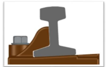
The chairs are fixed using a high tensile hexagon head screw with a flange under the head, so no washers are required.
