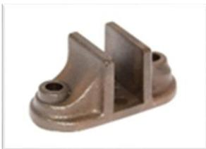
The bar rail chair is manufactured from a high-grade polymer, and is of a compact design of pleasing appearance, embodying many full-size features. If used with our plastic sleepers it has automatic gauge widening built in. If you want to lay a 5" gauge line as well in the smaller 10mm x 20mm bar rail then we can provide a packer which lifts the rail up.
